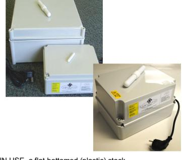
IN USE, a flat-bottomed (plastic) stock container is placed on the stirrer enclosure. The required amount of water (20 litres max. for the 6-240, 100L max for the 10-12 and 200L max. for the 15-12 version) is placed in the stock container along with the Teflon-coated magnetic follower. When the electrical power is switched on, agitation commences and a small vortex formed. Powder product added to the water will be kept in suspension during dosing.
